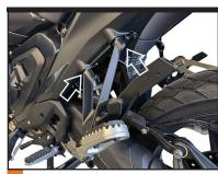
OPTIONAL: To provide sufficient working room, temporarily remove the Left side passenger footpeg using a T40 Torx socket wrench.
