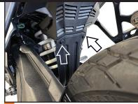
2 Remove the 2 plastic screws holding the rubber mudflap using a short Philips head screwdriver.
