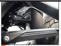
INSERT a New plastic screw in the upper LEFT side hole of the MudSling. Push and Screw it in until firmly seated.
